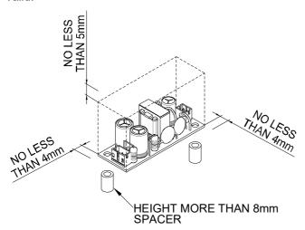
The CFM06SXXX and CFM06SXXX-E mounting holes are 1.5mm. Please allow 4mm side clearance from the components and all side of the PCB and CASE. Allow 5mm clearance above the highest parts on the PCB and CASE.
