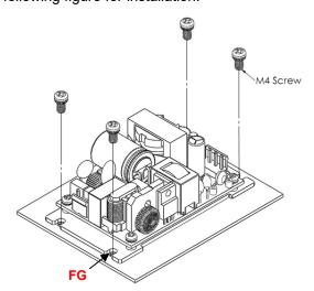
CFM130MXXX-B installation diagram
