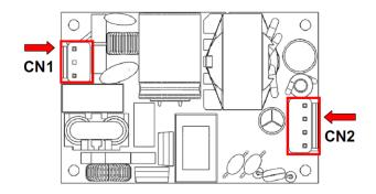
AC Input (CN1) DC Output (CN2) Wafer: TAIWAN KING PIN TERMINAL PVHI series or equivalent. Housing: JST VHR series or
