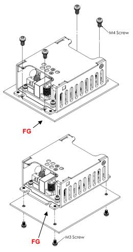
CFM130MXXX-C installation diagram
