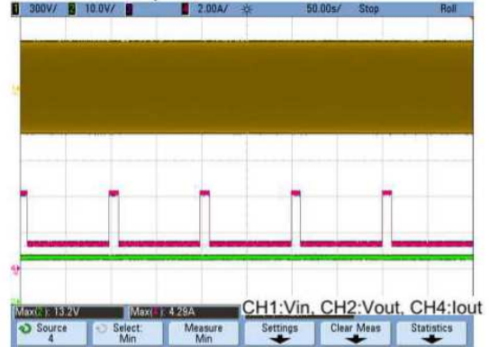
CH1:Vin, CH2:Vout, CH4:Iout Average Power:19.78W add external 33u / 400V capacitor to BC+& BC-.
