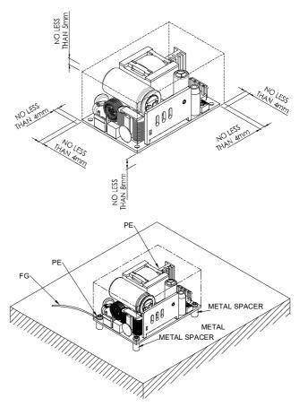
The CFM81SXXX-P mounting holes are 1.5mm. Please allow 4mm side clearance from the components and all side of the PCB. Allow 5mm clearance above the highest parts on the PCB.
