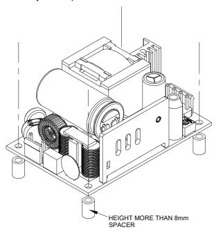
Please reserve 4mm space from the surfaces and the sides of PCB, especially from the solder surface, 8mm space is necessary. If the space is not enough, the specification of insulation and withstand will not be satisfied.
