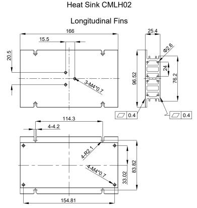
Heat Sink: 166\*96.52\*25.4 CMLH02 (G6621140202) Thermal PAD PCM02: PMP-P-400 164x75.2x0.25mm (G6135151B23) Screws: SMP4X8N M4\*8mm (G75A3300992) & Washer (G75A47A0832)
