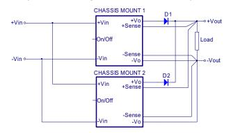
**Simple Redundant Operation Connect Circuit**
