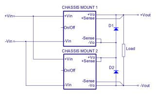
**Simple Series Operation Connect Circuit**
