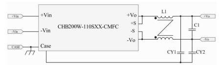
Connection circuit for EMI testing
