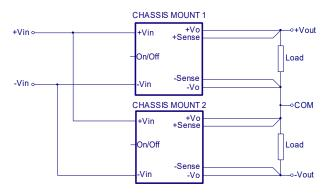
Simple ±Output Operation Connect Circuit
