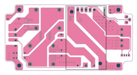
Figure 3 PCB layout bottom view
