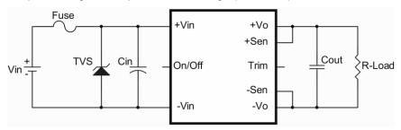
The external input capacitor (Cin) and transient voltage suppressor diode (TVS) are required if CQB50W12 series has to meet EN61000-4-4, EN61000-4-5.
