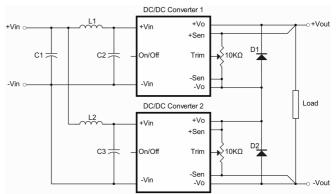
**Simple Series Operation Connect Circuit**
