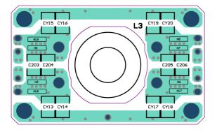
Figure 5 Output Filter PCB layout top view
