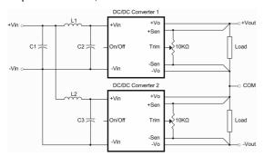
Simple ±Output Operation Connect Circuit
