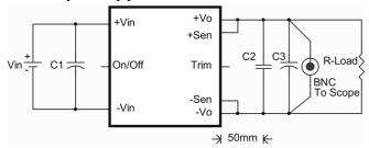
C1: 82uF/250V ESR<0.7Ω C2: 1uF/1206 ceramic capacitor
