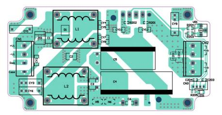
Figure 2 PCB layout top view
