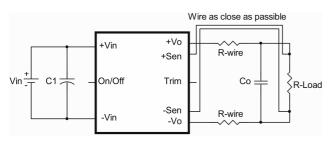
If the remote sense feature is not to be used, the sense pins should be connected locally. The +Sense pin should be connected to the +Vout pin at the module and the -Sense pin should be connected to
