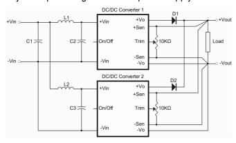
**Simple Redundant Operation Connect Circuit**
