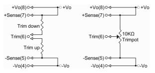
In order to trim the voltage up or down, one needs to connect the trim resistor either between the trim pin and -Sense for trim-up or between trim pin and +Sense for trim-down. The output voltage trim range is -20% to +10%. This is shown:
