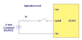
Figure 3 Recommended Application Circuit
