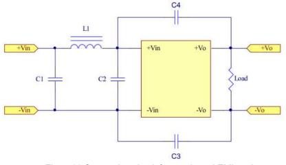
Figure11 Connection circuit for conducted EMI testing
