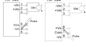
Figure 9 Using Probe to Measure Output Ripple and Noise
