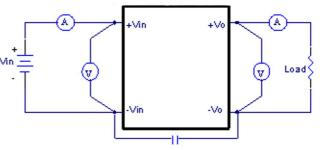
Figure 7 EC5SAW Series Test Setup NOTE:-Vin to -Vo With 470pF/250V Y1
