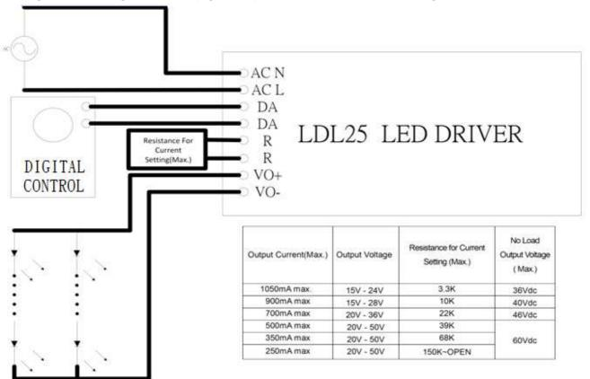
Figure 13 DIGITAL Dimming Function
