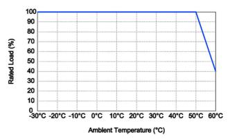
Figure 2. Typical Output power of LDL25 Series
