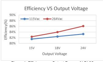
Figure 4. Efficiency vs. Output Power of LDL25 (to Output Current =1050mA)
