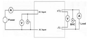
Figure 11. Output Voltage Ripple and Noise Measurement Set-Up
