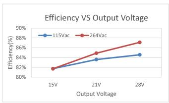
Figure 5 Efficiency vs. Output Power of LDL25 (to Output Current =900mA)
