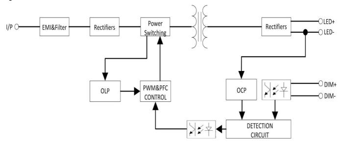
Figure 1. Electrical Block Diagram
