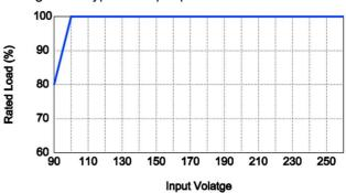
Figure 3. Typical Output Power De-rating of LDL25 (to AC input)
