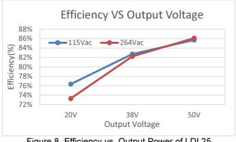
Figure 8. Efficiency vs. Output Power of LDL25 (to Output Current =350mA)
