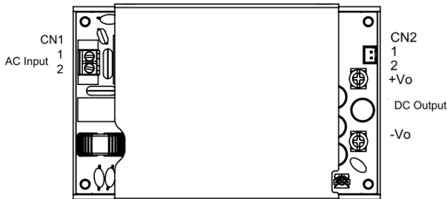
LFM420SXXXC Installation Diagram
